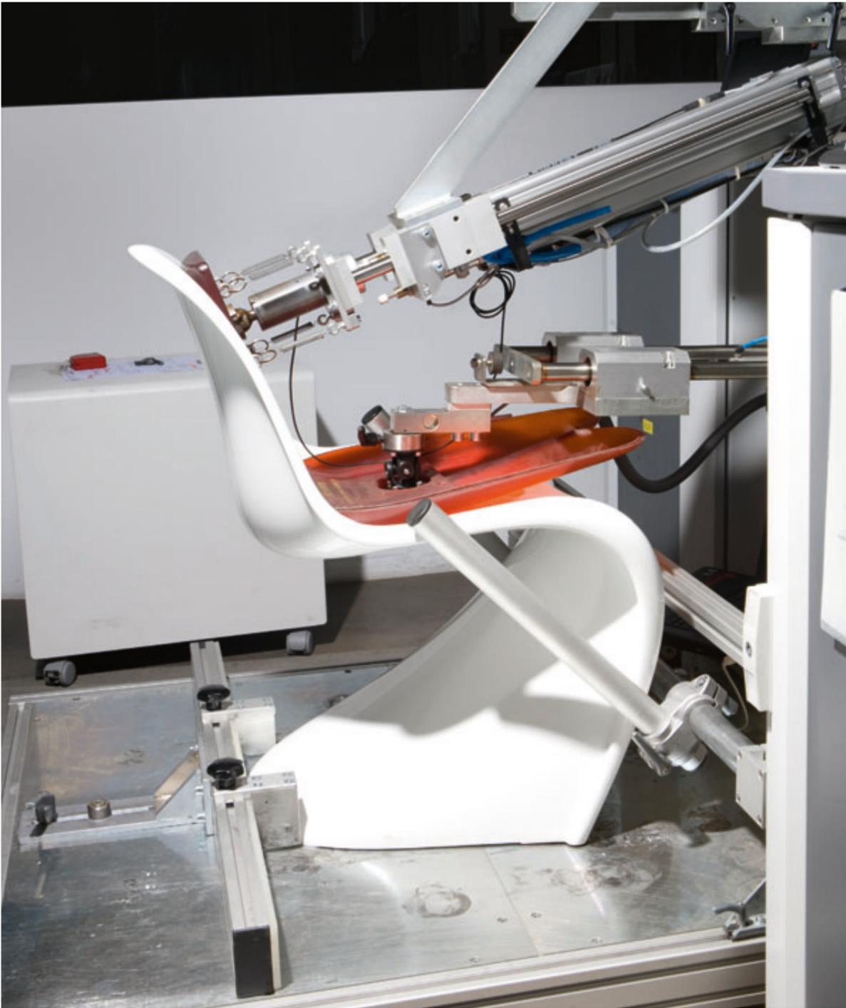
At the test centre on the Vitra Campus in Weil am Rhein, objects are subjected to quality controls. These tests are the basis for continuous improvements.
